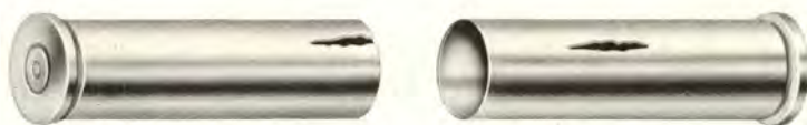
Cracks and splits around the neck or body are indications of deteriorated brass probably due to excessive reloading.
