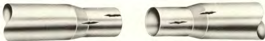
Cracks around the neck and splits in the body are indications of deteriorated brass probably due to excessive reloading.
